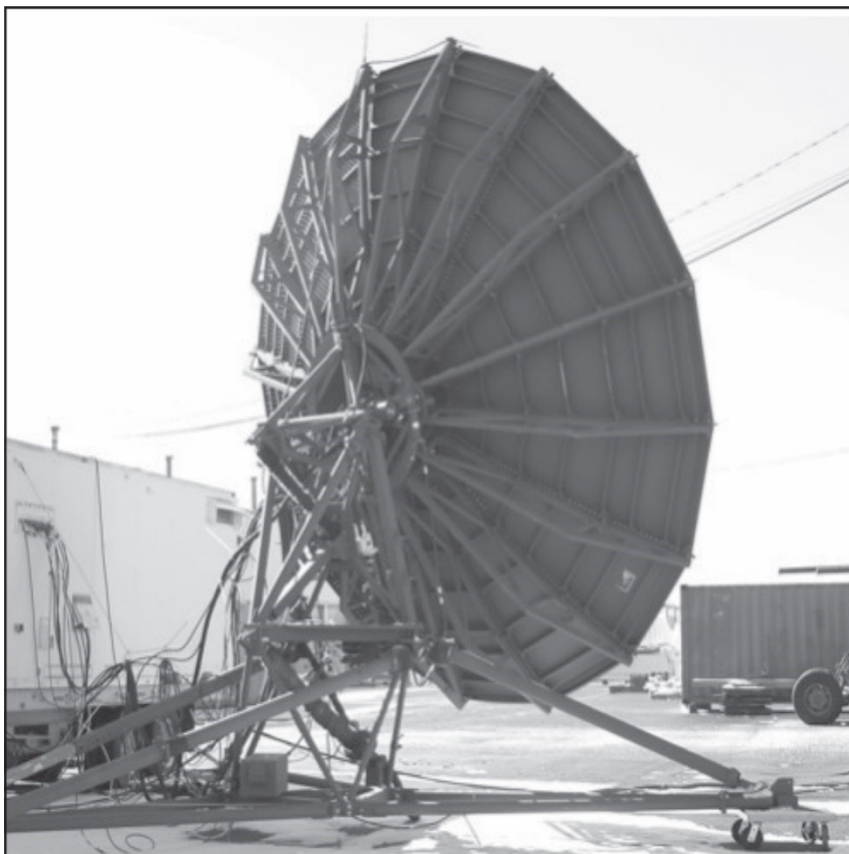
Figure A-7. AN/TSC-86A terminal
