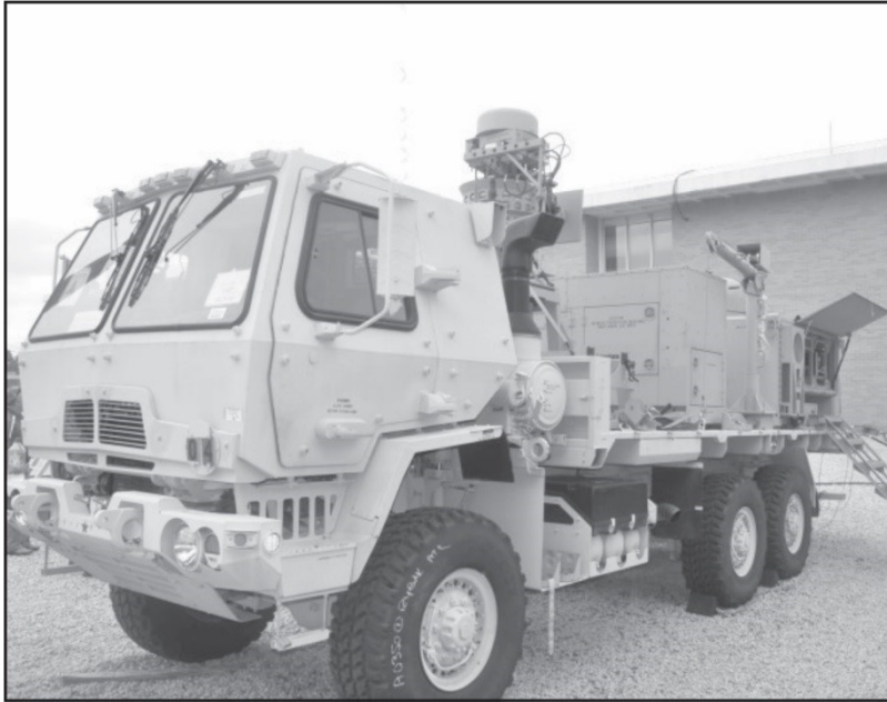
Figure A-15. Tactical communications node
