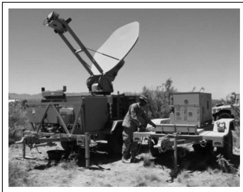
Figure 2-1. Satellite Transportable Terminal
